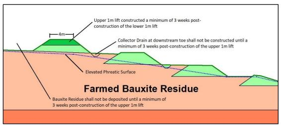
Figure 5.3: Stage Raise Construction Methodology (Source: Golder, 2021).
