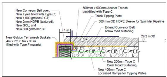
Figure 5.4: Typical Tipping Plate Section at SCDC (Source: AAL, 2021).
