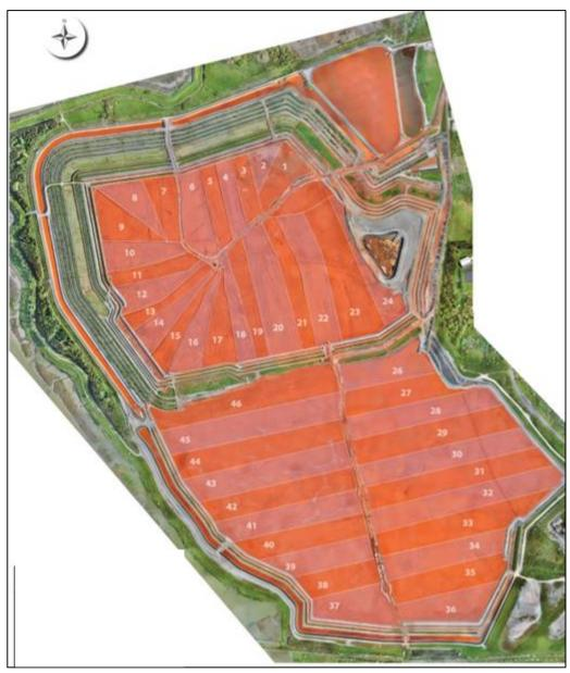
Figure 2.5: BRDA Layered Deposition Cell Layout (Source: Golder, 2021).
