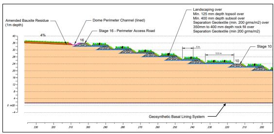
Figure 5.2: Section of Proposed BRDA Raise from Stage 11 to Stage 16 (Source: Golder, 2021).
