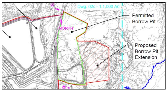
**Figure 5.6:** Permitted and Proposed Borrow Pit Extension (Source: Golder Associates – Drawing No. 02).
