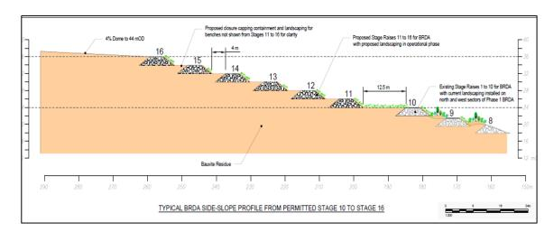
Figure 2.4: Typical BRDA Side-Slope Profile from Permitted Stage 10 to Stage 16
